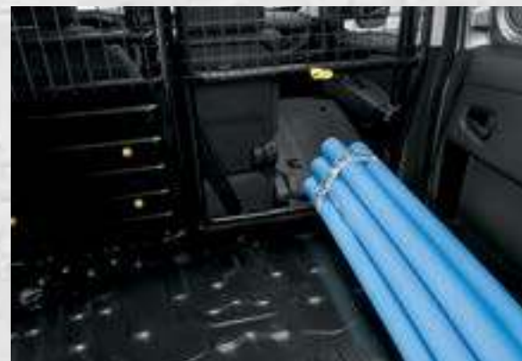
Multi functional partition for 3 seats configuration, removable on passenger side to accomodate long objects
