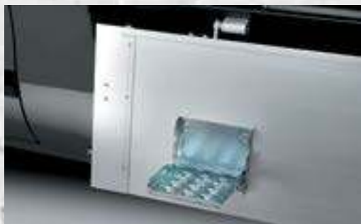
INTERNAL STEPS FOLDING INTO SIDEBOARDS
